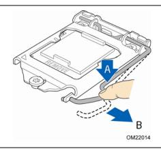
Figure 6. Unlatch the Socket Lever
